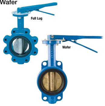
**Disc** – Disc edge is machined and polished 360° to assure leaktight shutoff while minimizing operating torque. Positive, disc-to-shaft connection is provided by stainless steel precision taper pins that are vibration proof.
